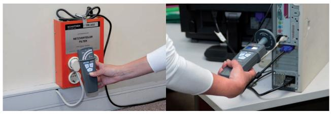
VX 0003 measuring while taking the user's presence into account.  VX 0100 and antenna measuring the electromagnetic fields in an office
