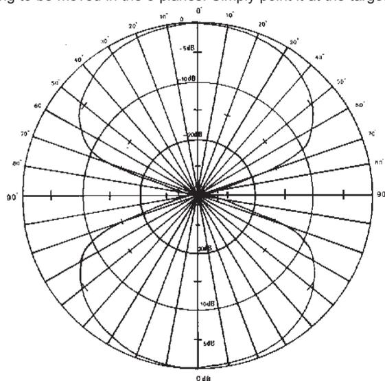
Because of the anisotropy of the measurement probe, during measurement in a given atmosphere, the aerial must be moved in all planes, along all axes (see figure) :
