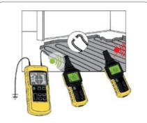
Fault detection in under-floor heating systems
