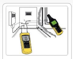
**Detection of metal water pipes**
