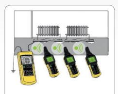
**Detection of metal heating ducts**
