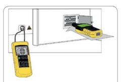
**Identification of fuses**Connect the transmitter to a power socket for simple identification of
