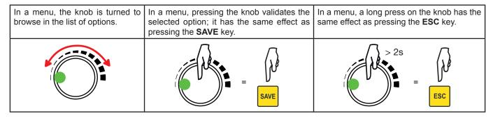
During a measurement in manual mode, it can be pressed to set the test current.
