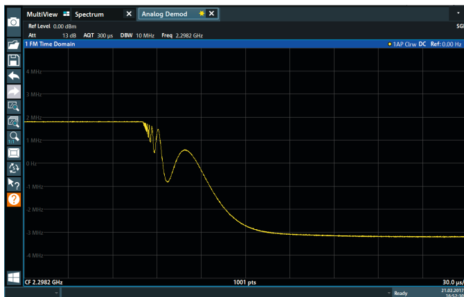
Frequency settling behavior of an oscillator.
