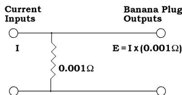
Insert the shunt's banana-plug outputs into the main voltage inputs on the multimeter (not the high ampere inputs). Then connect the current source to be measured to the shunt's input terminals (binding posts). *The multimeter will read the IR drop caused by the input current through the shunt.*
