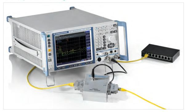
Compact test set consisting of the R&S<sup>®</sup>ESR EMI test receiver and the R&S<sup>®</sup>ENY41 coupling network for semiautomatic measurement of the asymmetrical disturbance voltage.
