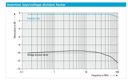
The typical insertion loss of the symmetrical circuit – measured with a line impedance of 100  $\Omega$  – determines the transmission bandwidth of the coupling network for the wanted signal; the typical voltage division factor (lower curve) is to be added to the measured voltage for the frequency range from 150 kHz to 30 MHz for comparison with the disturbance limit.
