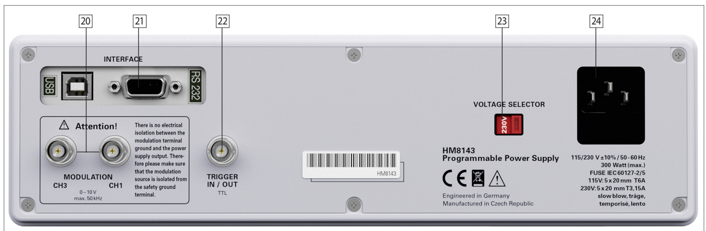
Fig. 2.2: Rear panel of the HM8143
