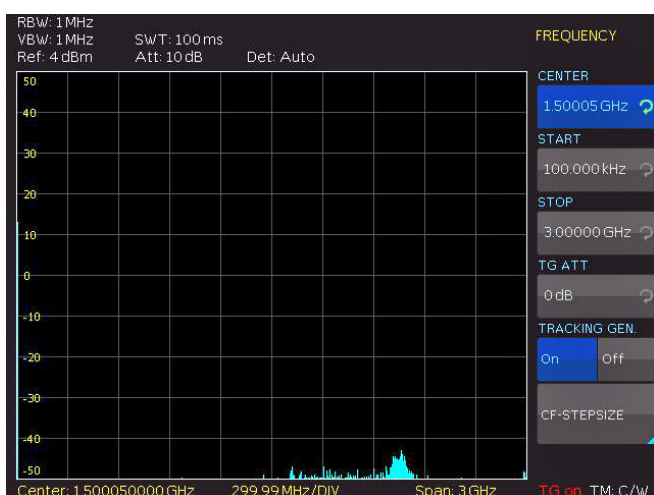
Fig. 6.11: Loosening of the RF cable completely
