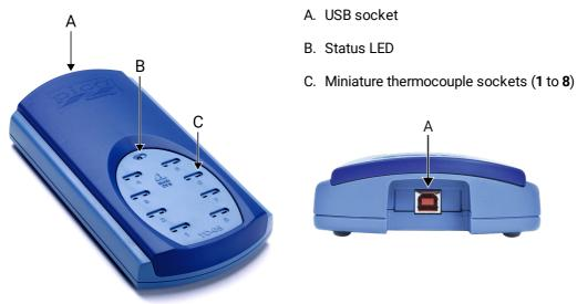
Install the PicoLog software before connecting a TC-08 for the first time.
