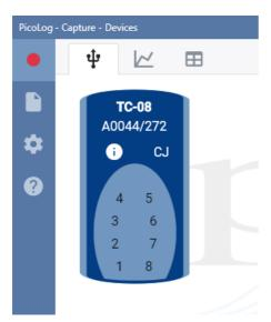
1. Select the channel corresponding to the location you chose for the thermocouple. The channel setup dialog will then display, allowing you to configure the channel. You can type in a channel **Label** and choose a channel **Color**, **Sample interval** and **Input type** (thermocouple type). You also have an advanced option to set **Custom scaling**:
