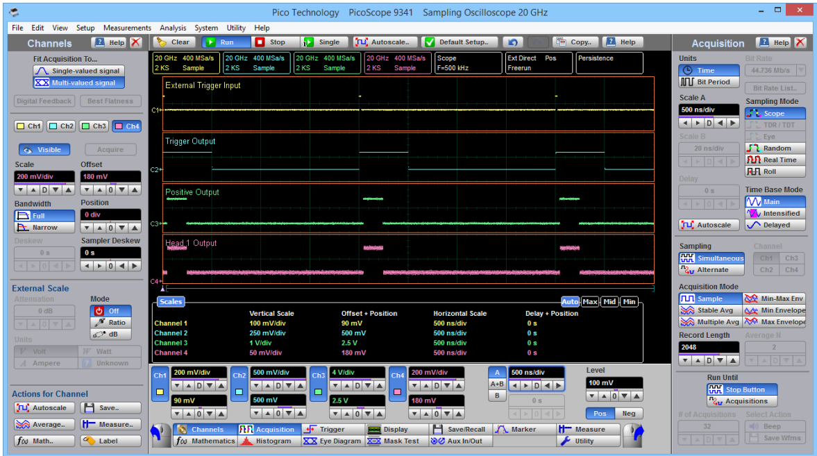
Timing diagram for external triggered mode (2 \mu s period of external signal)
