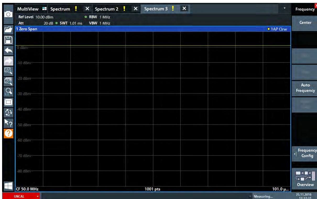
Figure 6-7: Time domain display of the calibration signal
