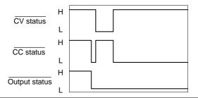
CC MODE: Output turned off The diagram below shows the output status lines when the output is turned off in CC mode.
