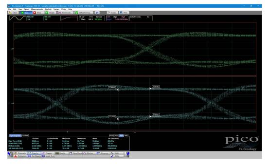
Eye diagram analysis can display data including: bit rate, period, crossing time, frequency, eye width, eye amplitude, mean, area and jitter RMS. Also shown on the graph are left and right RMS jitter markers. These measurements are selectable from within the Eye Diagram side menu and are listed on screen below the graph.
