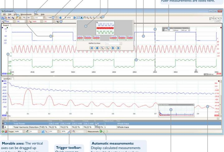
axes can be dragged up and down. This feature is particularly useful when one waveform is obscuring another. There's also an **Auto Arrange Axes** command.
