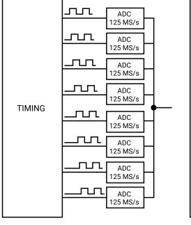
and display signals up to 200 MHz with a high sampling rate, or lower-speed signals with 256 times more resolution than typical 8-bit oscilloscopes. Resolution enhancement—a digital signal processing technique built into PicoScope 6 can further increase the effective vertical resolution of the scope to 20 bits.
