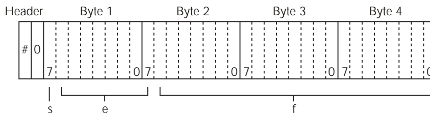
Figure 18-2 IEEE-754 single precision data format (32 data bits)
