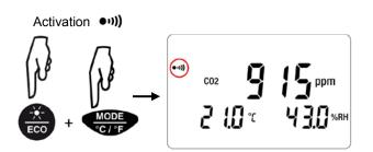
First press the **ECO** key, then, while keeping it pressed, press the **MODE** key.
