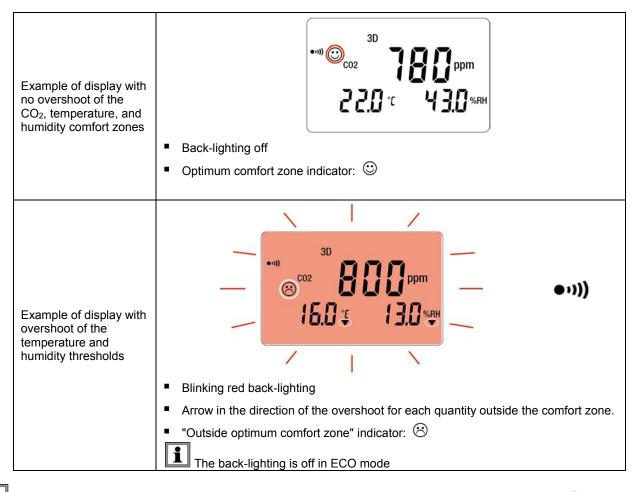
For the **1D** and **3D** modes, if the buzzer is active, it will sound intermittently upon the appearance of the 😕 symbol.
