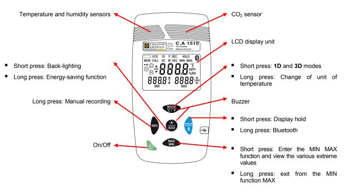
On the keys, the function written above the line is invoked by a short press, the function written below the line by a long press.
