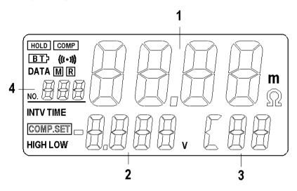
1 Displays the resistance measured or the resistance limit settings of the comparator function
