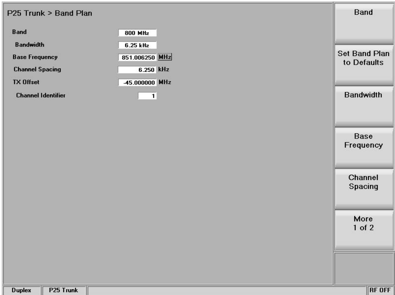
Figure 3.2.8.5-4 P25 Trunk Band Plan submenu
