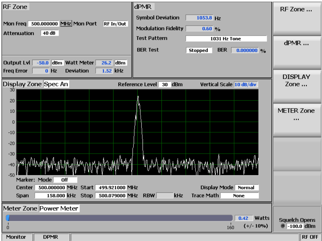
Figure 3.2.8.9-1 Main screen in Monitor Mode after selecting dPMR Test Mode
