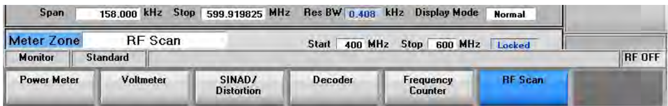
Figure 3.2.6-2 Meter Zone submenu after Select Meter soft key press
