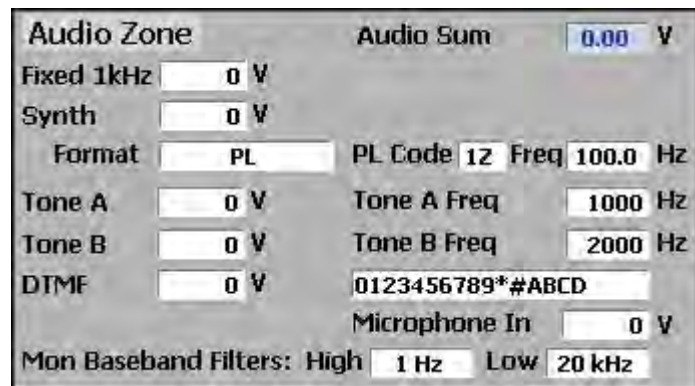
Figure 3.2.4-2 Audio Zone display with the R8000 in Monitor Mode
