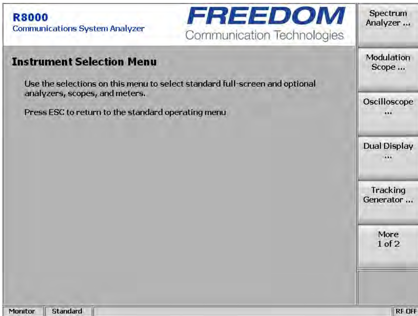
Figure 3.2.7-1 Submenu after pressing Instrument Navigation key
