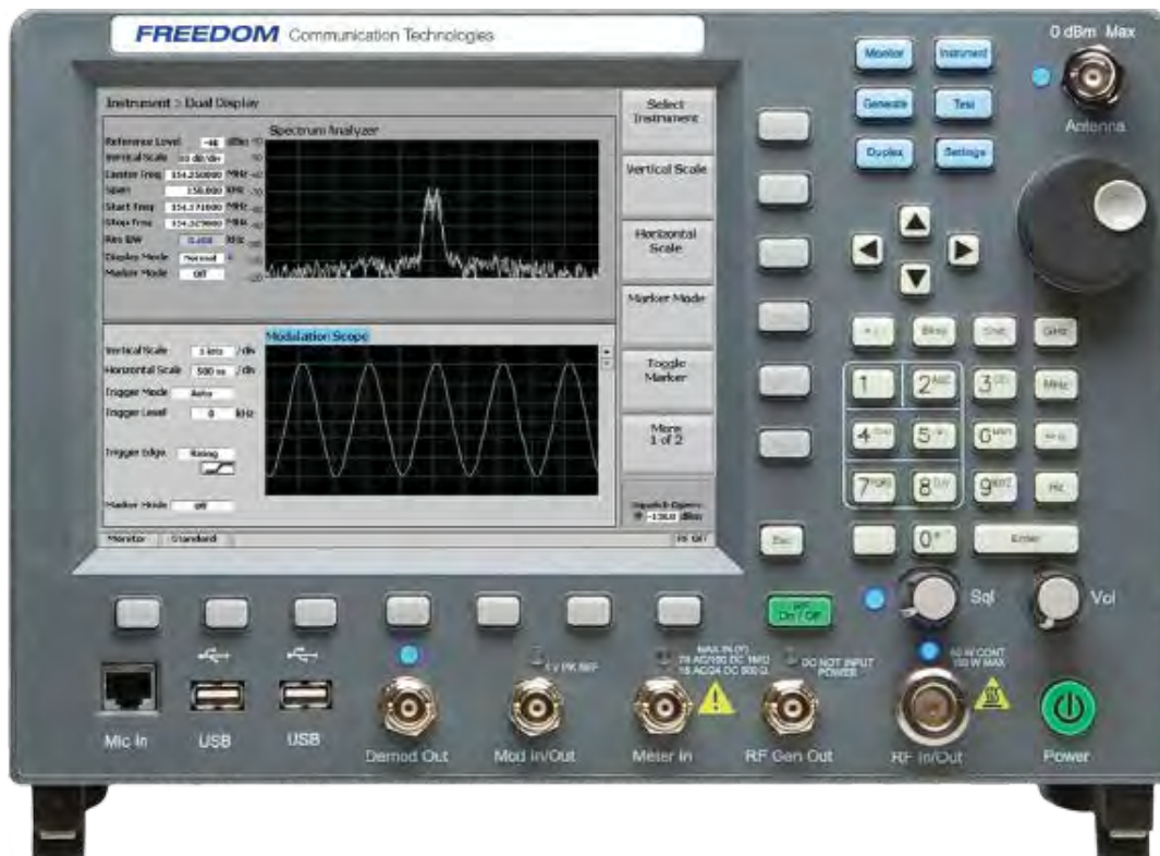
Figure 2.1-1 Front Panel Controls, Indicators, and Connectors
