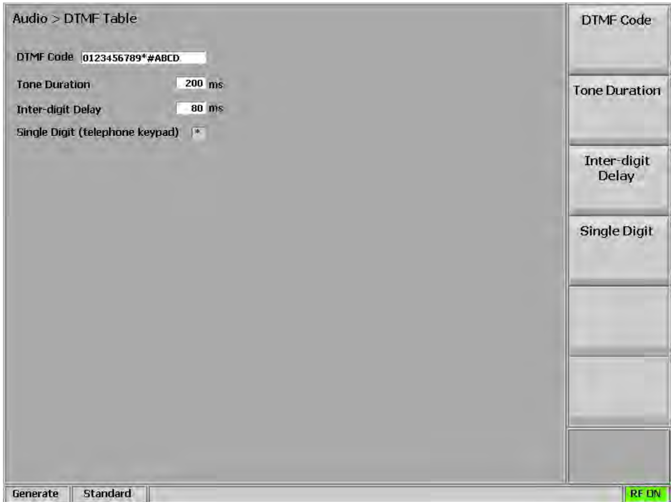
Figure 3.2.4.2-2 DTMF Table providing additional code sequence control.
