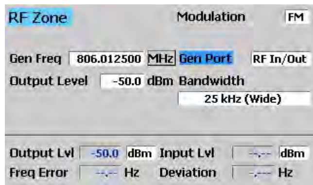
Figure 3.2.2-1 RF Zone display area showing Generator Mode data with RF Level Offset enabled
