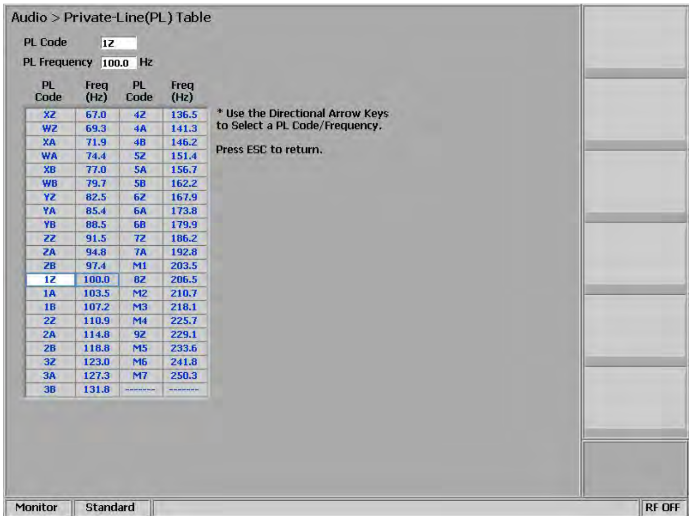
Figure 3.2.4.3-1 PL Table showing highlighted entry code
