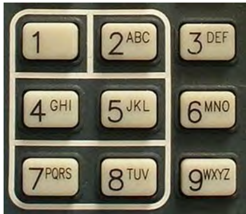
Figure 3.1.2-1 Outline around Numeric Keypad Hot Keys
