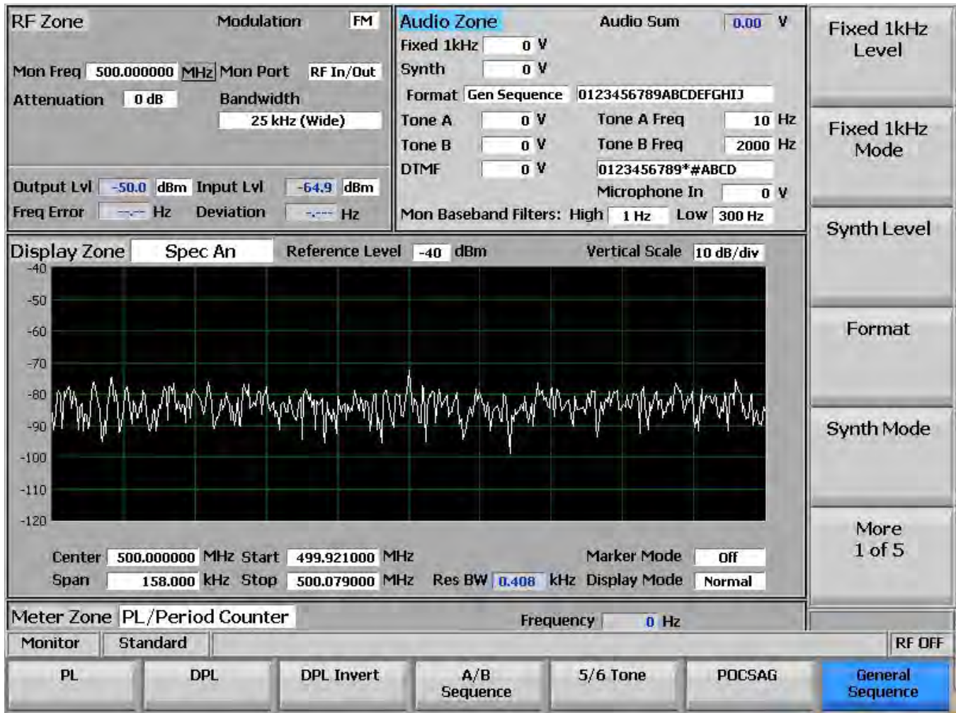
Figure 3.2.4.2-1 Format submenu in Audio Zone
