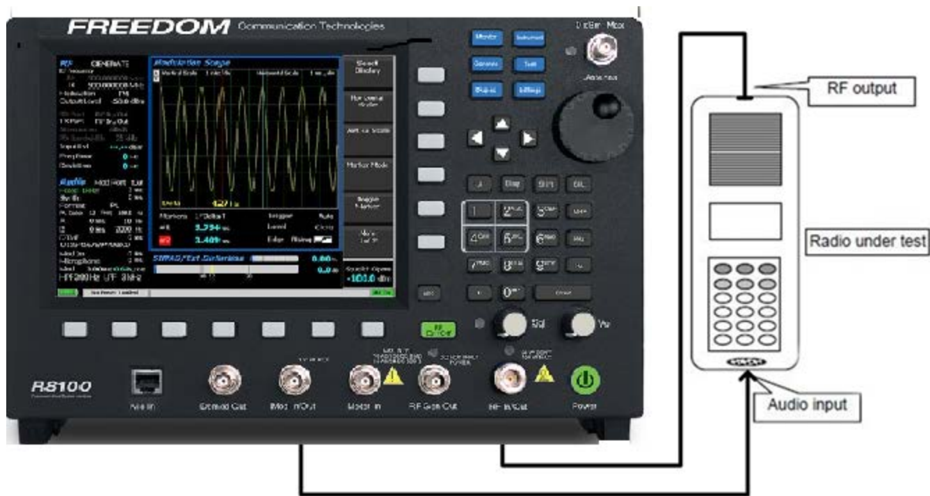
Figure 5.1.1-1 Setup for FM Transmitter testing
