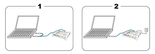
**Note:** If you connect or disconnect the AC adaptor while the oscilloscope is in operation it will restart automatically and any unsaved data will be lost.
