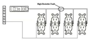
In this example there is a High Resistance Fault between the  $2^{nd}$  and  $3^{rd}$  receptacle. The Voltage drop increased from the  $2^{nd}$  to the  $3^{rd}$ . The high resistance was identified as a poor connection between the two devices.
