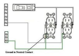
SureTest® Circuit Analyzer can detect a false ground condition within 15 feet of a receptacle under test or within 15 feet of the panel.
