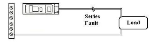
*Glowing Contact, or High Resistance Series Arcing Fault*<sup>3</sup> is defined as the abnormally high resistance in a wire, wire termination, wire splice of and type of connection, resulting in reduce current flow and excessive heat at the fault.
