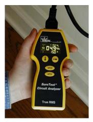
Voltage drop at a 12, 15, or 20 ampere load can be easily taken by simply plugging the SureTest ® into a receptacle and performing the Voltage drop test.
