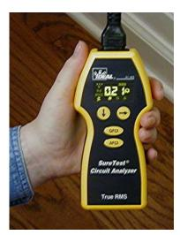
The IDEAL SureTest® can measure the resistance of the Line, Neutral, and Ground conductors. This can be very helpful when trying to locate a high resistance fault in a branch circuit.
