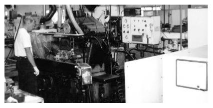
As shown above, industrial machines containing variable speed drives can cause a variety of costly power quality problems.
