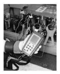
The versatility of the IDEAL Power Analyzer means simultaneous recording of all parameters for extended periods of time.
